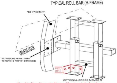
Floor plates / base plates can be either one of these shown in the above diagram
